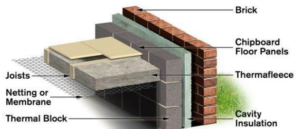
If the flooring comprises open floorboards, you could install a breather membrane on the top side of the Thermafleece to avoid a build-up of dust and debris on top of the insulation.
