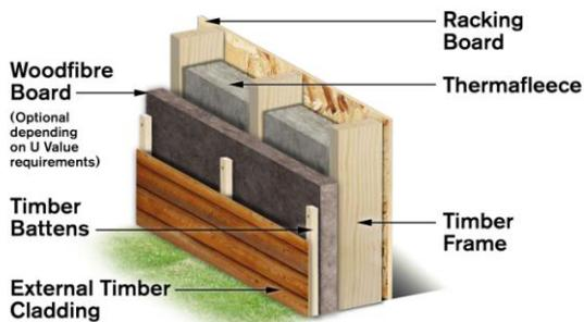
Unlike traditional timber frame systems, the racking board is positioned to the inside of the timber frame. The external insulation attached to the timber frame maintains the frame above the dewpoint temperature reducing the risk of condensation. Additional benefits include low environmental impact, lightweight structure and improved insulation and airtightness.
