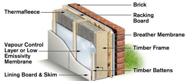
Fix VCL to the warm side of the insulation to reduce the risk of interstitial condensation. The addition of vapour impermeable materials must be correctly detailed and materials must be completely sealed to ensure that no moisture can penetrate into the structure.
