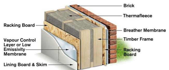
The twin frame system ensures that reduced thermal bridging occurs within the construction helping to maximise insulation performance. By using two 89mm structural timber frames, the width of the construction can be varied to achieve specific insulation performance.
